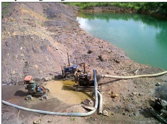
Lead Mining Pit Drained of Over Flooded Water (Source: Survey)
