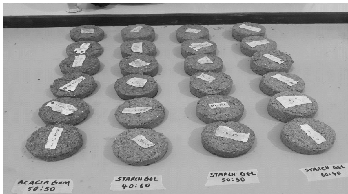
Fig. 1: Samples of Fabricated Briquettes with Different Proportions of Binders
