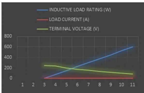
Figure 8: Load Output characteristic with Shunt and Series Capacitor of 25µf and 70µf.
