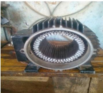
Figure 2: Stator Frame
