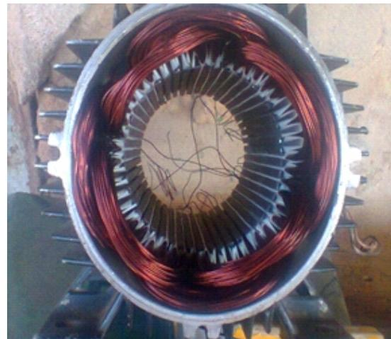
Figure 5: Complete Stator Wound Three Phase Four Pole Induction Motor
