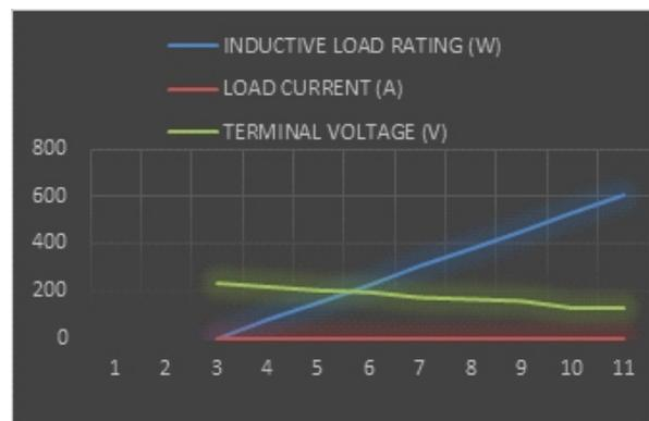
Figure 9: Load Output characteristic with Shunt and Series Capacitor of 25µf and 90µf.
