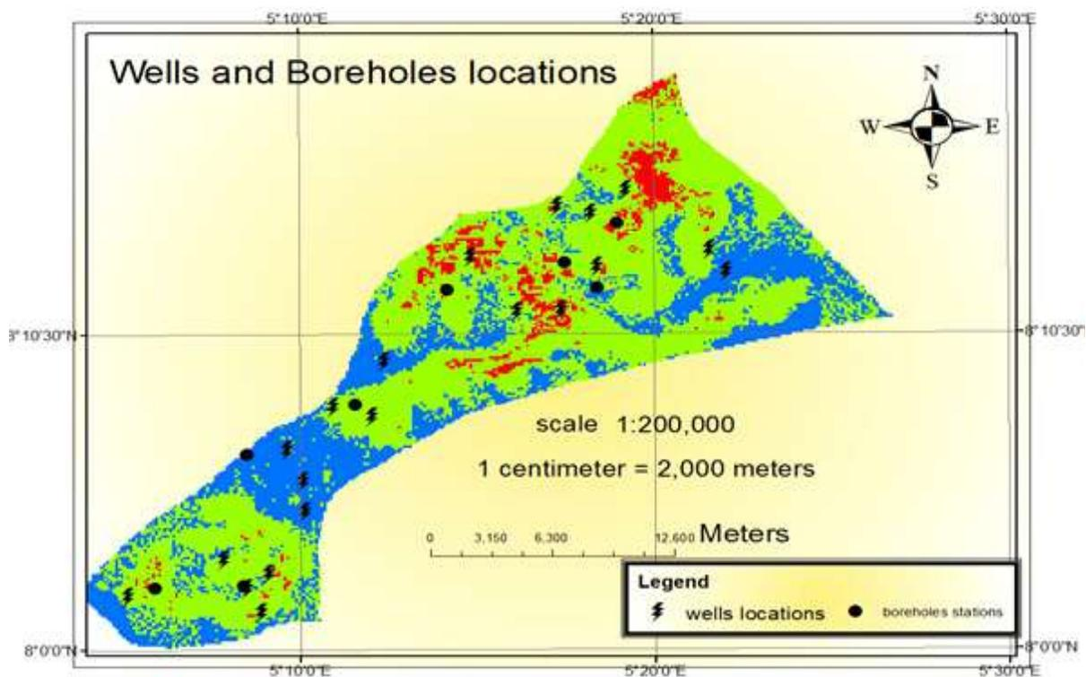
**Figure 2: Boreholes and wells Locations Superimposed on Groundwater Potential Zone Map (Souce: Agboola, 2019; with modification)**
