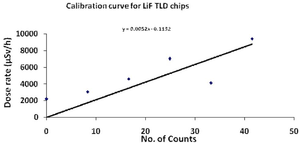
Figure Calibration curve of LiF TLD chip with Cs-137 gamma radiation source
